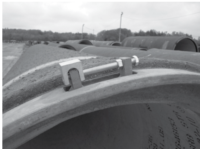
single bolt of Snap Ring restrained joint in unlocked position
