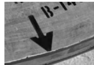
long side of a beveled pipe
