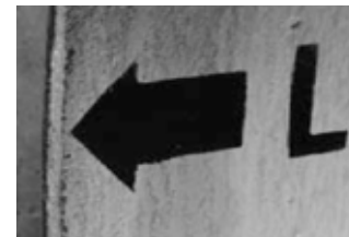
long side of a beveled pipe
