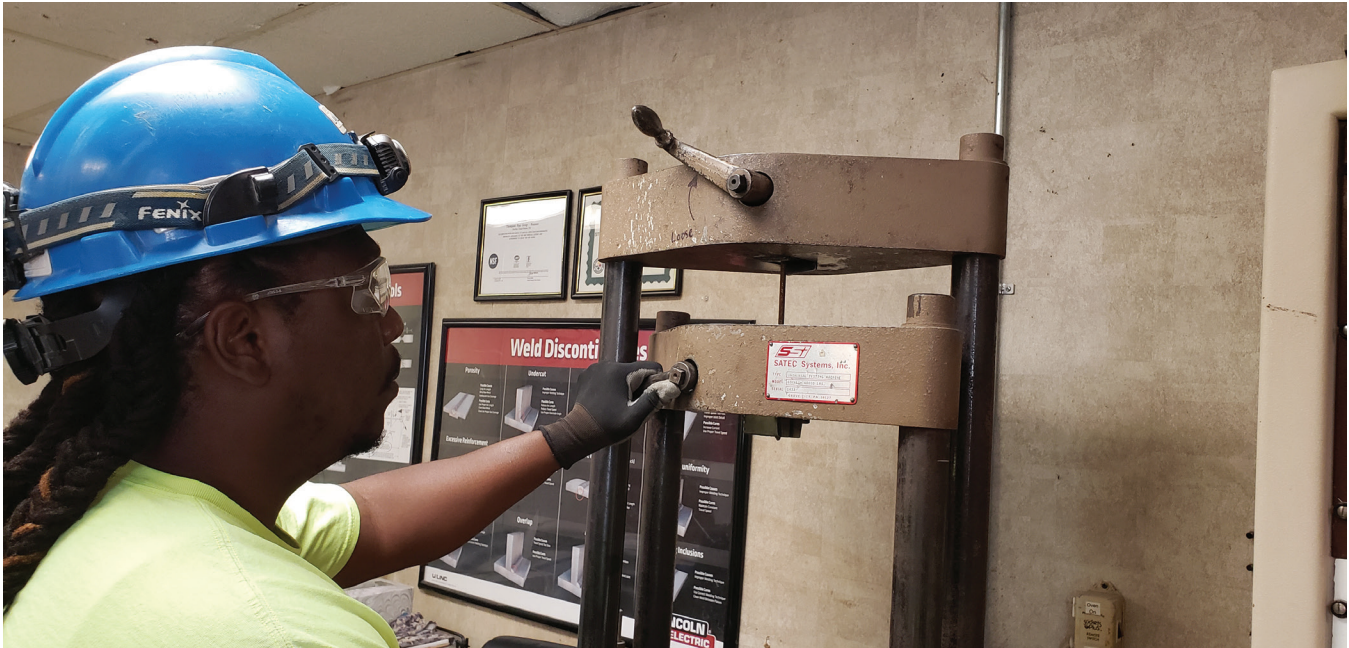
Prestressing wire is tested for tensile strength and ductility characteristics.
