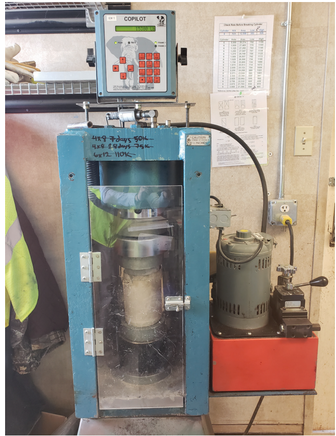
This test specimen of concrete used in the manufacturing of a pipe undergoes a standard concrete compression test. Test specimens are made daily and are cured under the same conditions as the pipe.
