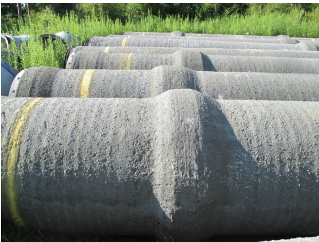
Figure 1: Raised mortar coating skids on L-301 pipe
