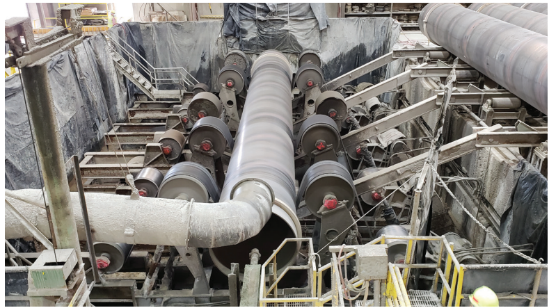
Concrete is centrifugally cast within the steel cylinder to form the pipe's concrete core.
