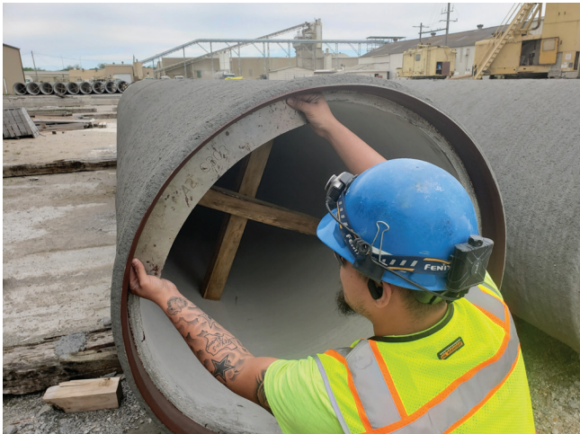
The Thompson Pipe Group team of Quality Assurance inspectors receives extensive training on monitoring in-process and finished pipe quality factors, such as checking roundness of pipe joint rings.
