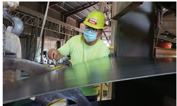
A quality control technician checks cylinder steel thickness. Each heat of cylinder steel must also meet ASTM standards referred to in AWWA C301 and C303 for acceptable yield strength.
