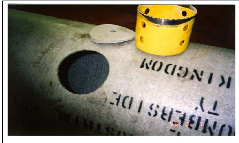
Figure 6: Alternative cutter with closely spaced teeth
