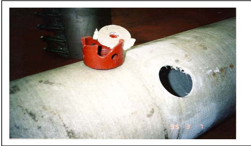
Figure 7: Unsuitable cutter with widely spaced teeth. This cutter has few widely spaced teeth and tears glass fibers from the laminate.
