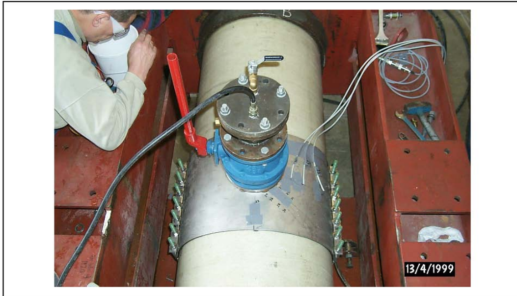
Figure 2: Pressure testing of sleeve and valve assembly
